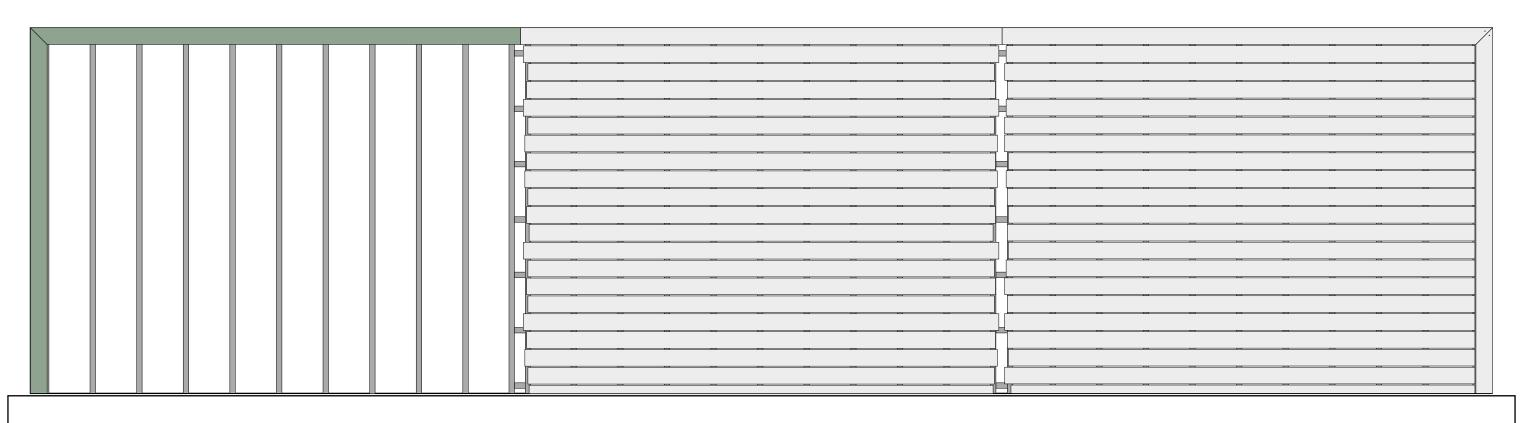
Step 5: Cut the last framing boards to length, mitre and install.
