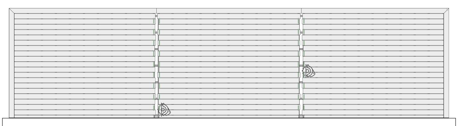
Step 7: With the boards fully fastened, use a guide or straight edge and your circular saw to trim to length.
