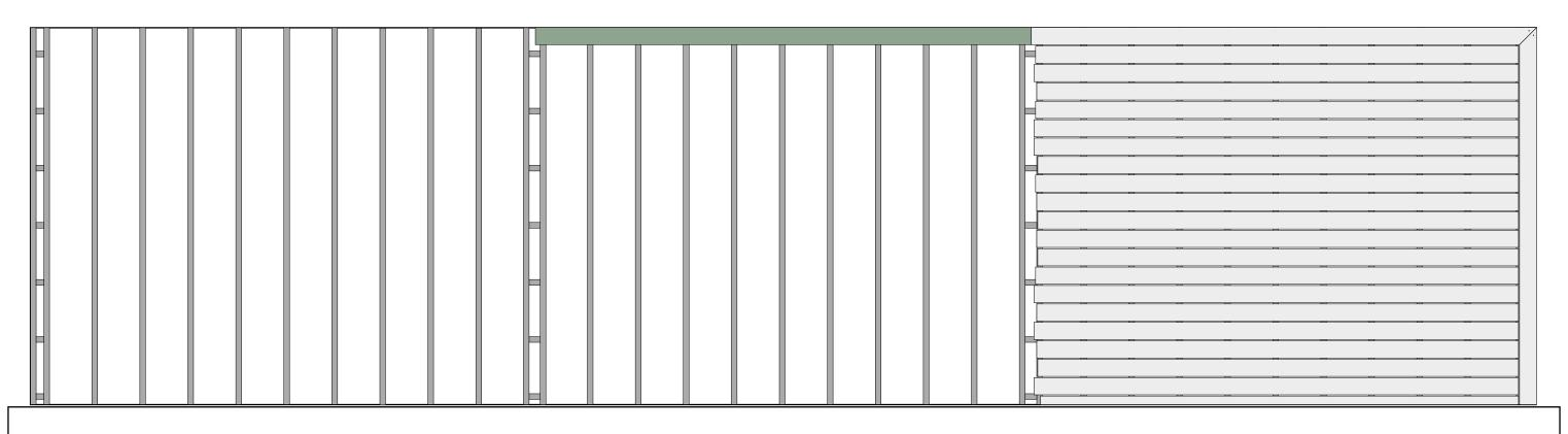
Step 3: Cut the framing board for the middle section to length and install.
