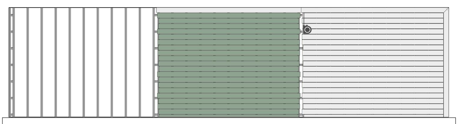
**Step 4:** Cut all the boards for your second section slightly over-length. Install the boards from the outside moving in towards the house.
