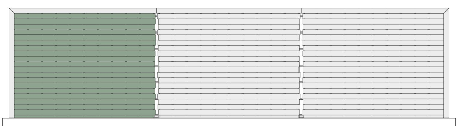
**Step 6**: Cut all the boards for your last section slightly over-length.
